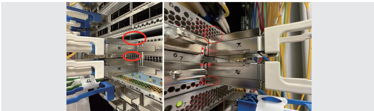
Figure 2: Examples of 400ZR Cooling Mechanism
