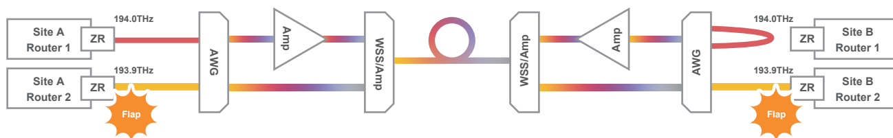
Figure 6: Issues with IP over DWDM
