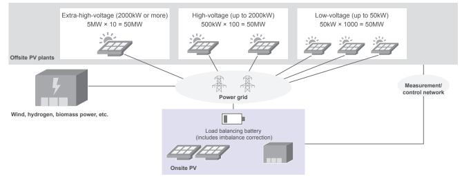
Figure 3: Carbon Neutral Data Center Reference Model
