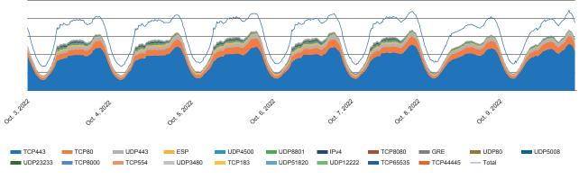
Figure 10: Breakdown of IPv4 Traffic by Source Port Number
