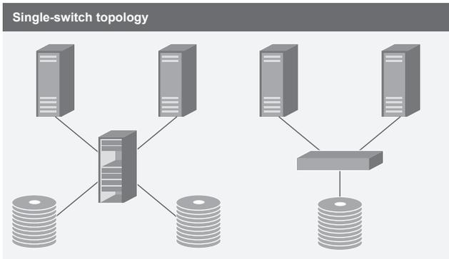
Figure 5: FC Fabric Topology with a Single Switch
