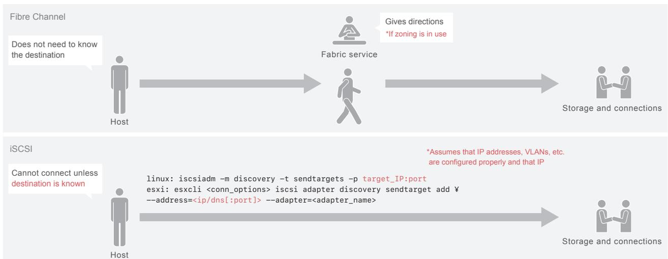
Figure 7: Difference between FC-SAN and IP-SAN Connections
