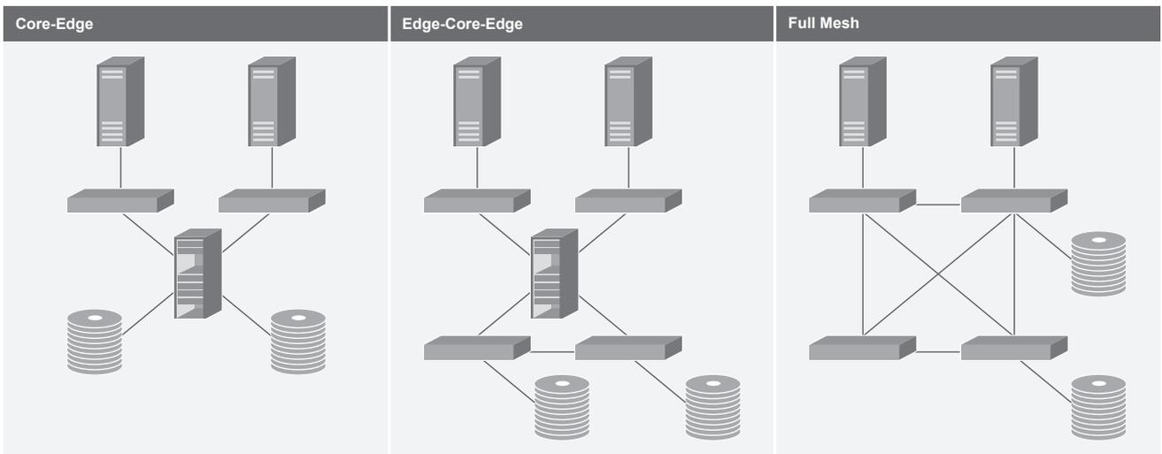
Figure 6: FC Fabric Topology with Multiple Switches
