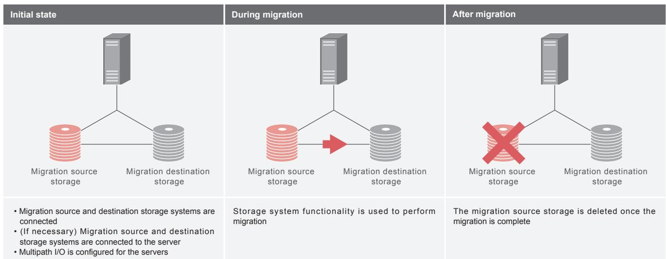
Figure 10: Migration Using Storage System Functionality
