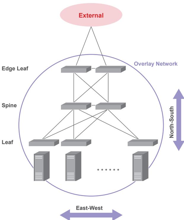
Figure 2: Overlay Network in a Large-scale Environment
