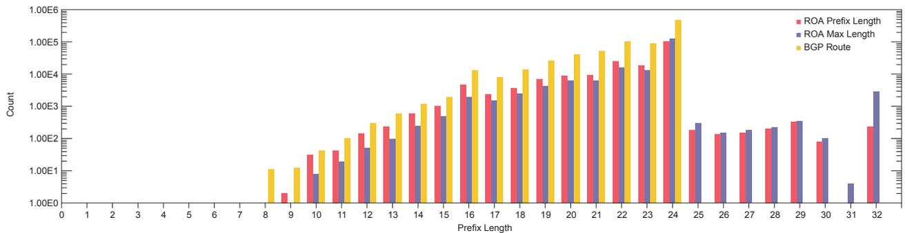
Figure 3: ROA Prefix Lengths and BGP Prefix Lengths (IPv4)
