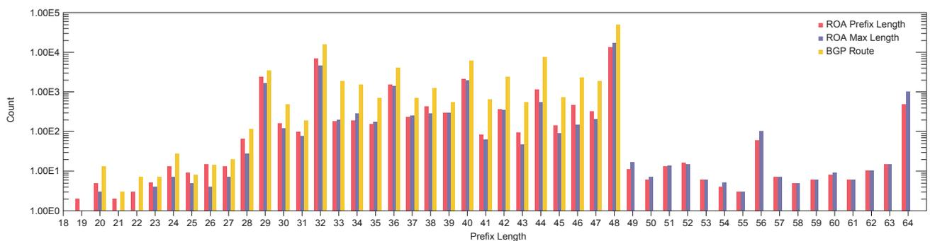
Figure 4: ROA Prefix Lengths and BGP Prefix Lengths (IPv6)
