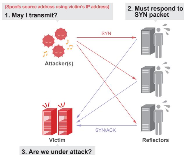
Figure 4: Overview of a SYN/ACK Reflection Attack
