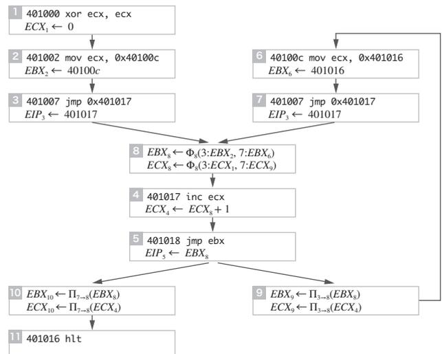
Figure 8: PSA Form: Insertion of  $\Pi$ -functions
