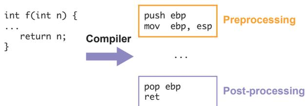
Figure 3: Preprocessing and Post-processing of Functions
