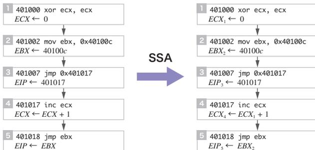
Figure 6: SSA Form: Up to the end of the first (A) call
