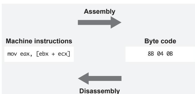
Figure 1: Disassembler
