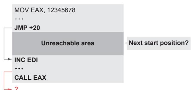
Figure 2: Recursive Descent Disassembler
