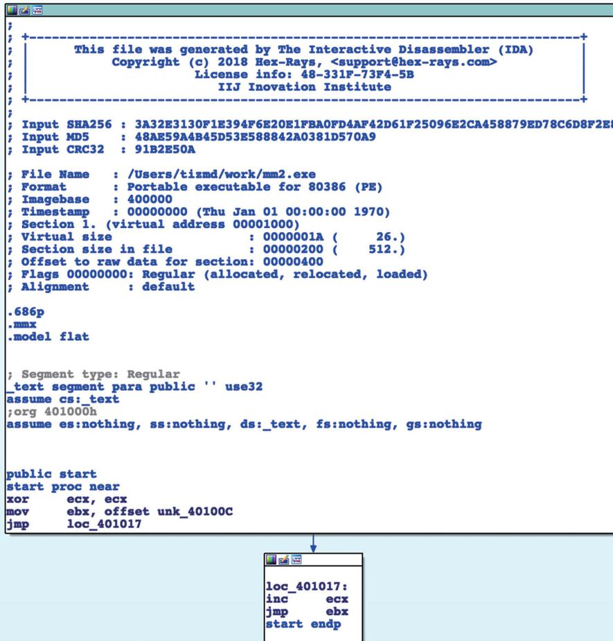
Figure 5: Example of Disassembly in IDA Pro
