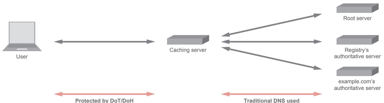
Figure 2: Scope of Transport Encryption
