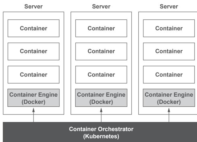
Figure 1: Container Engines and the Container Orchestrator
