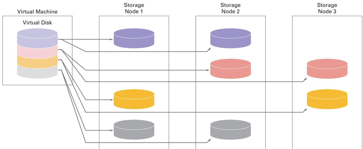
**Figure 3: Conceptual Diagram of UKAI Virtual Disk and Actual Data Storage**
