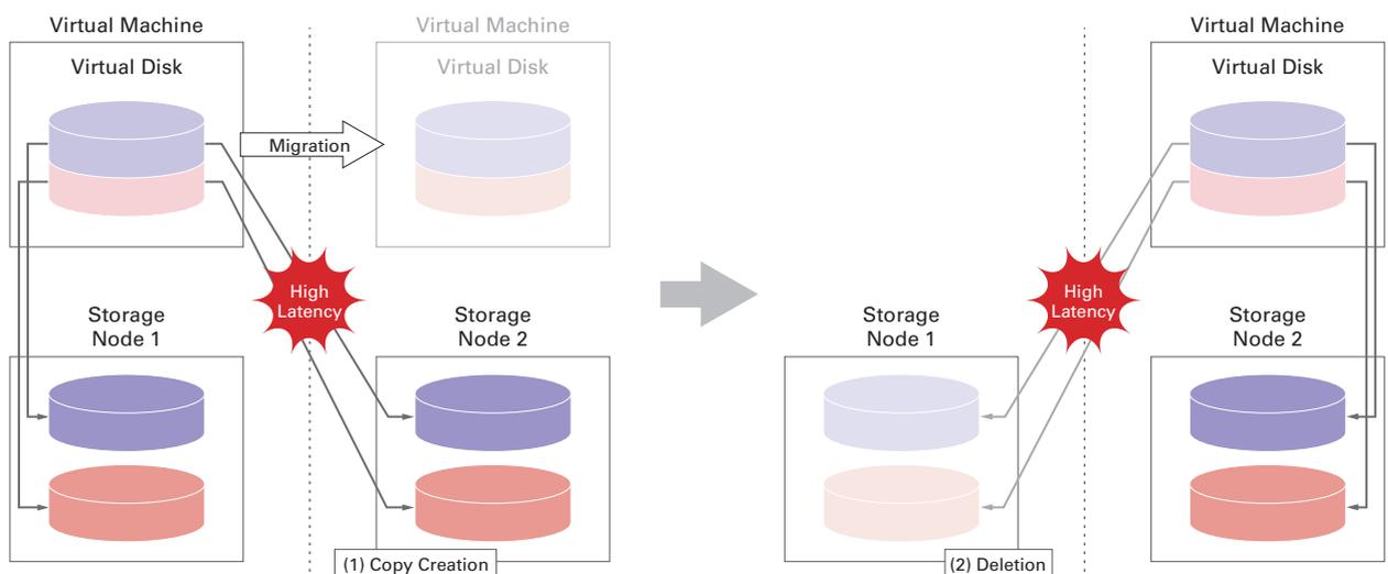
**Figure 4: Virtual Disk Relocation**
