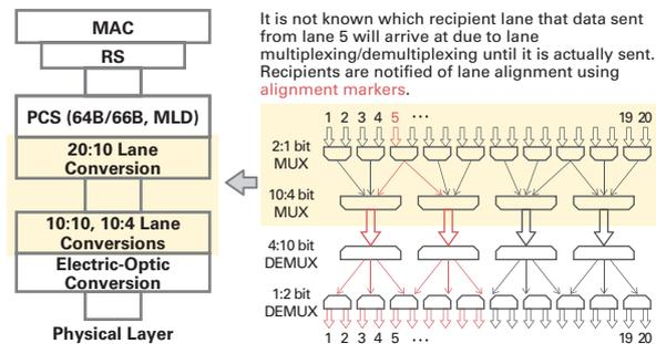
Figure 4: Relationship Between Sender/Recipient Lanes During Lane Multiplexing/Demultiplexing
