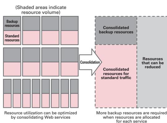
Figure 3: Backup Resource Reduction due to Website Consolidation
