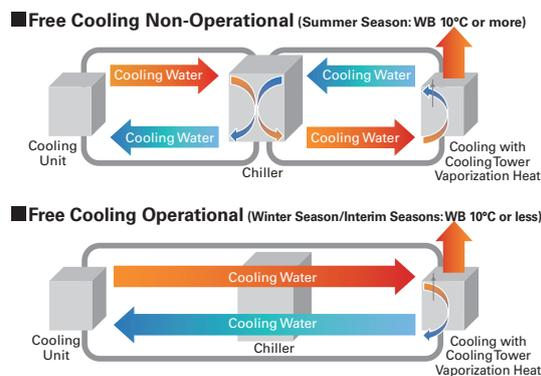
Figure 1: The Principles of Chiller-less Water Cooling Systems
