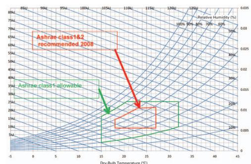
Figure 5: ASHRAE Recommended Temperature and Humidity Levels for Data Centers
