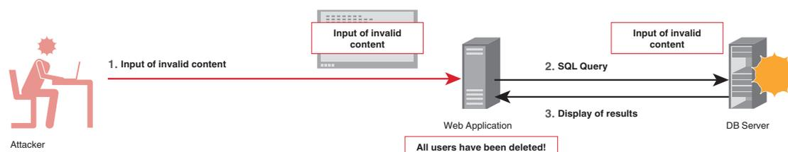
With a SQL injection attack, invalid input is transferred to a DB through the Web application, resulting in unintended behavior.
