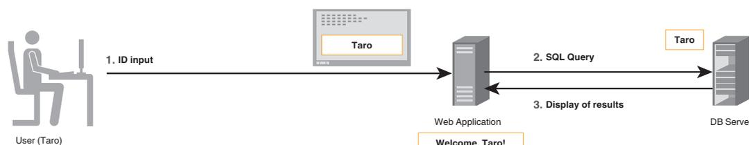
Under normal access conditions, user input is transmitted to a DB through a Web application, and the relevant content is produced.
