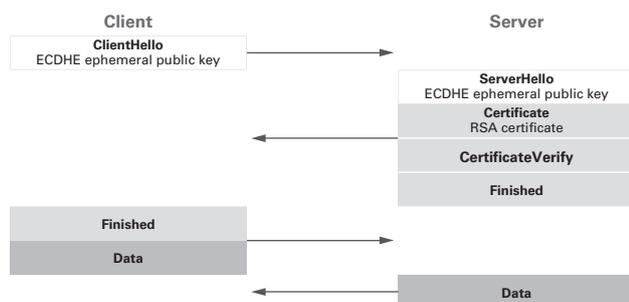
Figure 3: TLS 1.3 Full Handshake TLS\_ECDHE\_RSA\_WITH\_AES\_128\_GCM\_SHA256
