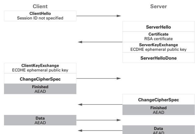
Figure 2: TLS 1.2 Full Handshake TLS\_ECDHE\_RSA\_WITH\_AES\_128\_GCM\_SHA256
