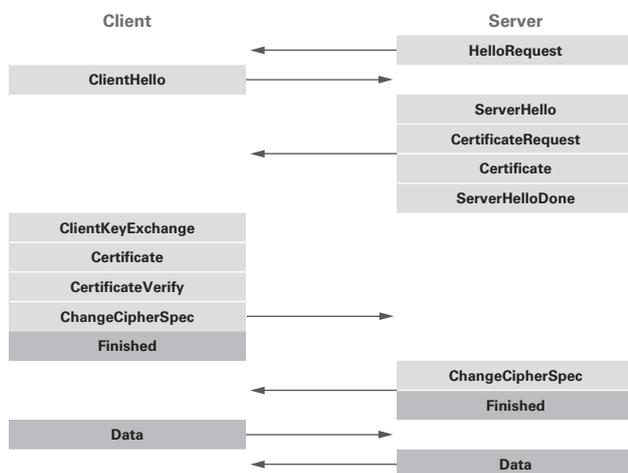
Figure 8: Certificate-Based Client Authentication Using TLS 1.2
